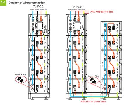
Note: It is not recommended to install a DC circuit breaker between the battery system and the hybird inverter system, If you want to install a DC circuit breaker with rated working voltage grearer than 1000V and rated working current greater than 63A, do not operate the DC circuit breaker with power on, otherwise the machine may be damaged.
