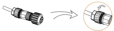
5. Align the groove of male terminal with the convex of female terminal, then tighten the bush in male terminal.
