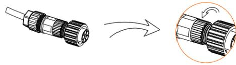
4. Tighten the screw of the back shell and the cable nut.
